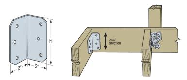
FIGURE 7: ML Dimensions and Typical Installation
