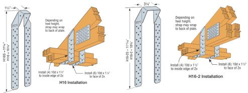
FIGURE 2: H16 and H16-2 Dimensions and Typical Installation
