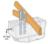
FIGURE 3: H16 Typical Installation to Masonry
