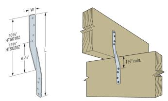
FIGURE 5: HTSQ Dimensions and Typical Installation
