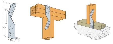
FIGURE 4: TSP Dimensions and Typical Installations
